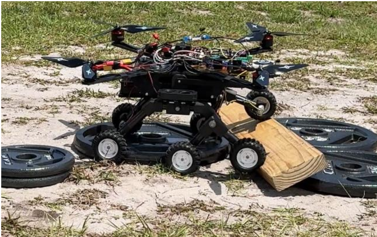
Figure 131: Terrain Test Showcasing Rocker-Bogie
