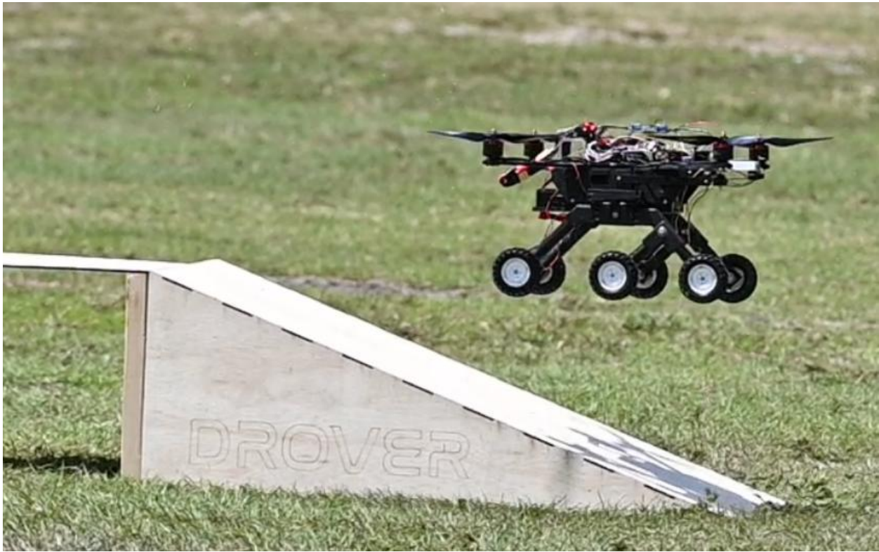
Figure 130: Obstacle Course Test (Right before landing on 20-degree incline)
