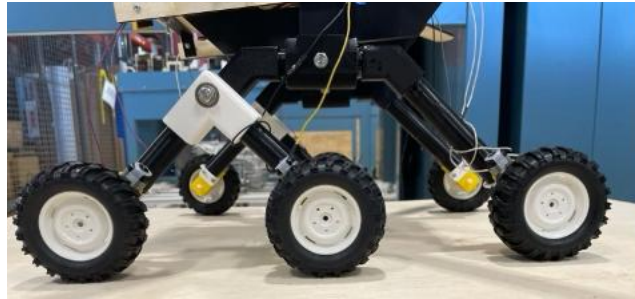
Figure 62: Leg assembly in prototype
