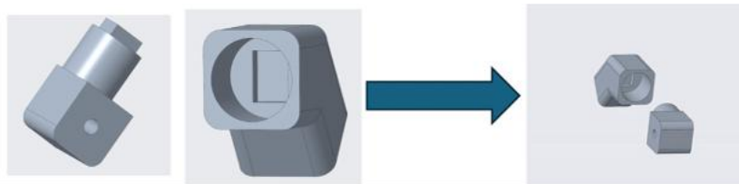
Figure 50: CDR Leg connection attachments
