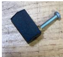
Figure 139: Onyx shaft with brass heat insert
