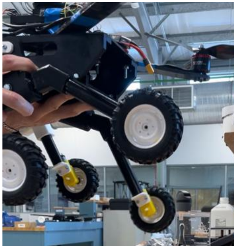
Figure 59: Rocker-bogie mechanism (one wheel up and the opposite down as intended)
