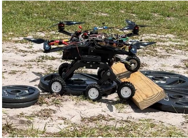
Figure 42: Rocker-Bogie Suspension System
