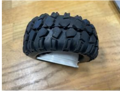
Figure 141: Wheels after zero-point turning
