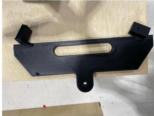
Figure 148: Broken Plate Support
