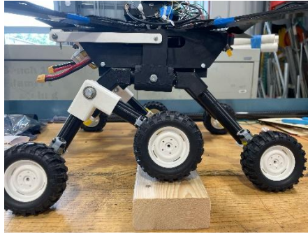
Figure 66: Pin Connection climbing 4.5 cm obstacle
