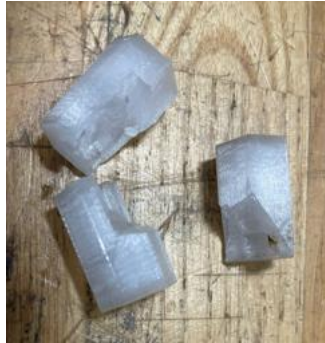
Figure 140: Broken Polycarbonate Shafts
