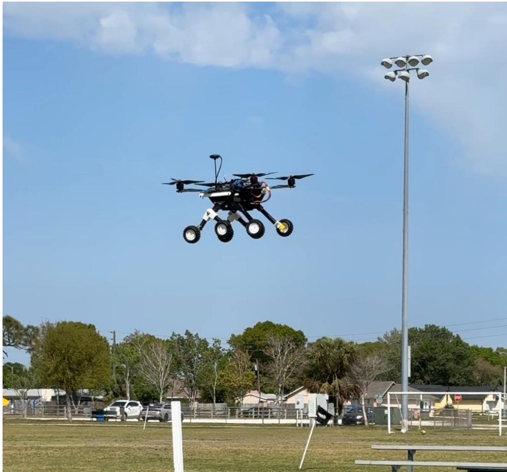
Figure 127: Flight Test With Leg Structure
