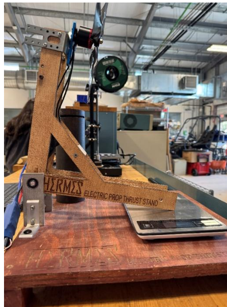
Figure 115: Thrust Test Setup
