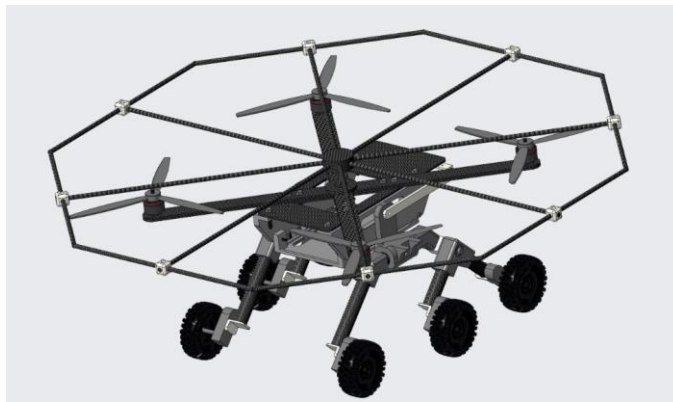
Figure 158: Initial CAD Draft for "drone cage" concept
